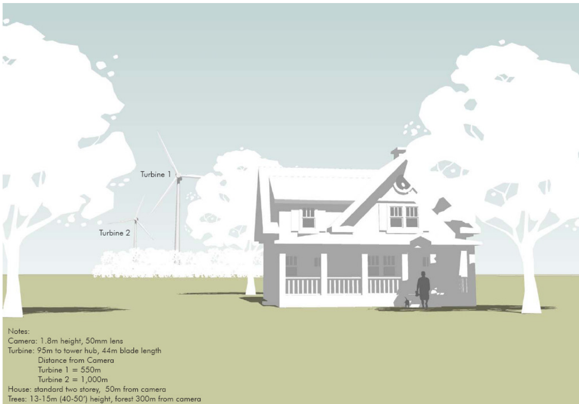
Visual Aid 2 Wind Turbine Scale Schematic, with trees
