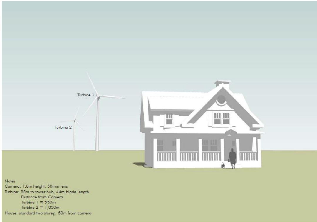
Visual Aid 1: Wind Turbine Scale Schematic
