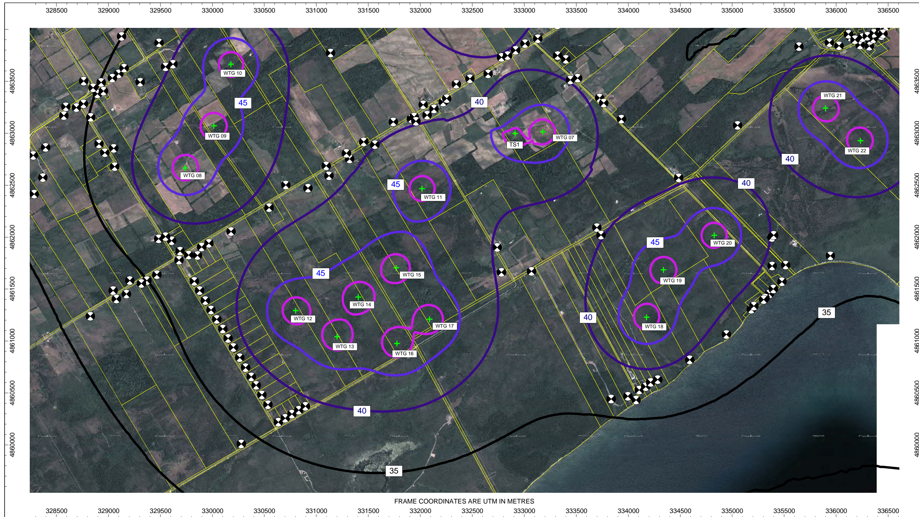
Figure 5b: Predicted Sound Levels, Leq [dBA], Southwest wpd Canada Corp. - White Pines Wind Project, Prince Edward County, Ontario Sound Level Grid Height Calculated at 4.5m
