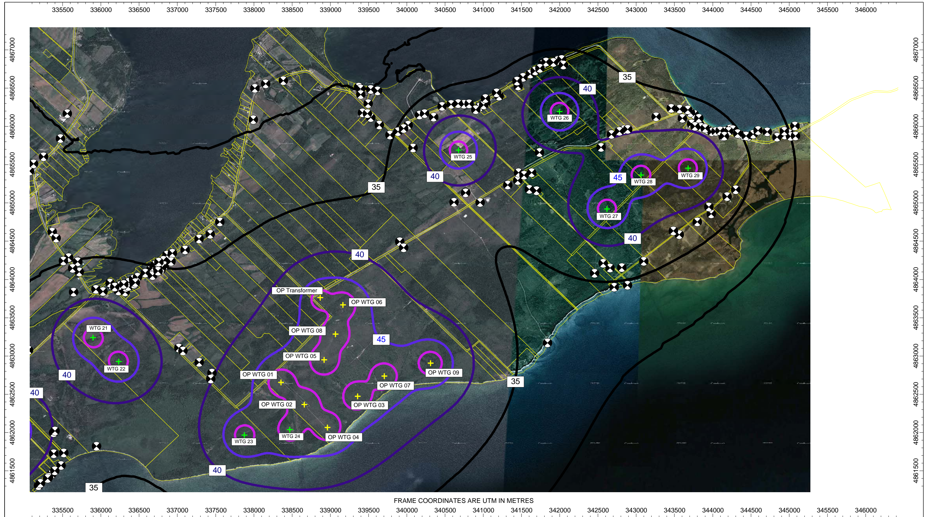
Figure 5c: Predicted Sound Levels, Leq [dBA], East wpd Canada Corp. - White Pines Wind Project, Prince Edward County, Ontario Sound Level Grid Height Calculated at 4.5m
