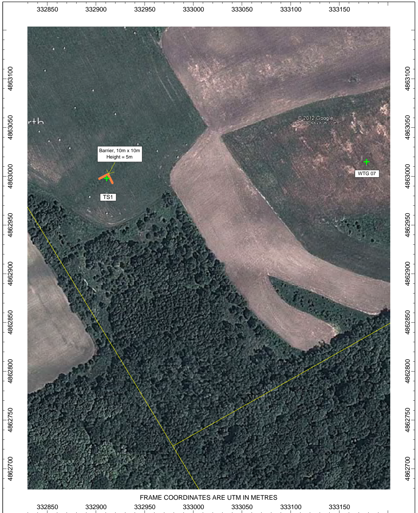
Figure 3: Proposed Transformer (TS1) Acoustic Barrier wpd Canada Corp. - White Pines Wind Project, Prince Edward County, Ontario
